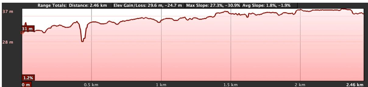
Figure 3.4. Elevation profile from WB7ABP (left) to WW6D (right). Note that with antenna heights of 50' at WB7ABP and 30' at WW6D this is a line of sight path except for suburban structures. Courtesy Google Earth.
