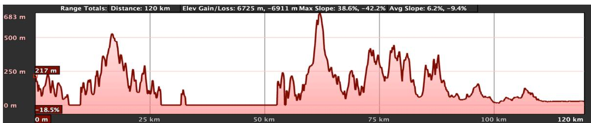
Figure 3.10. Elevation profile from WB7ABP (left) to KFS (right), the flat path is over seawater of San Francisco Bay. Courtesy Google Earth.
