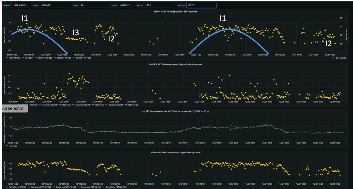
Figure 3.19. Time series of SNR with sun elevation, spectral spread, noise level and signal level for WB7ABP at KA7OEI-1 (Northern Utah SDR site).
