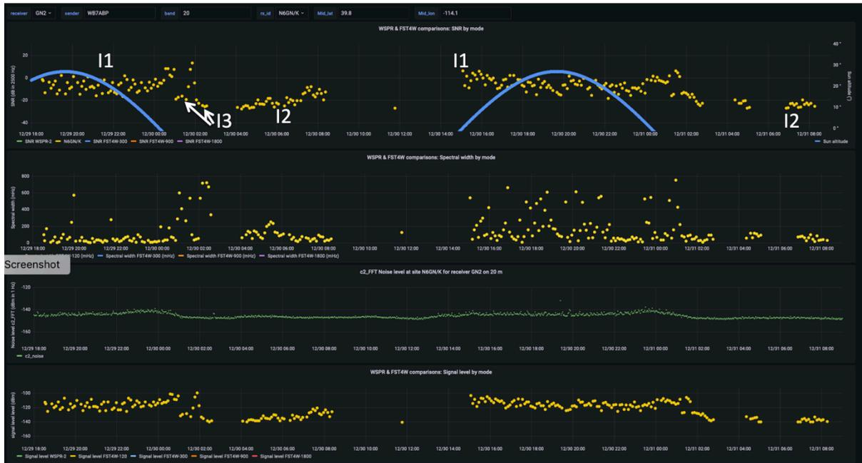
Figure 3.21. Time series of SNR with sun elevation, spectral spread, noise level and signal level for WB7ABP at N6GN/K.
