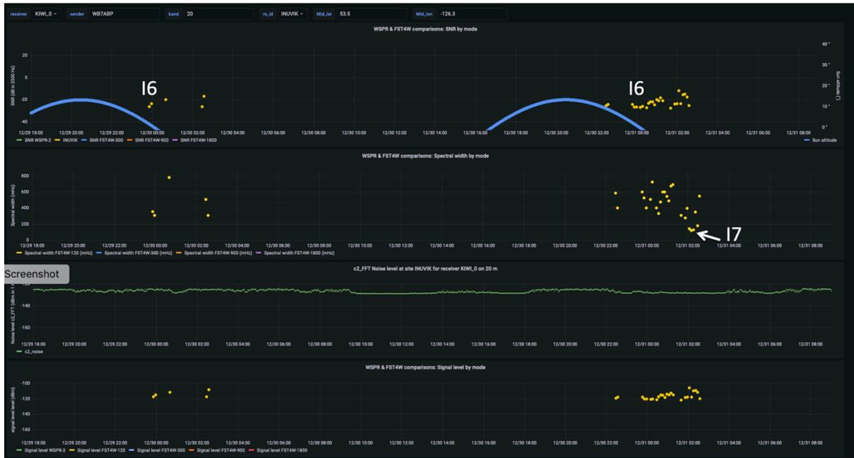
Figure 3.27. Time series of SNR with sun elevation, spectral spread, noise level and signal level for WB7ABP at INUVIK.
