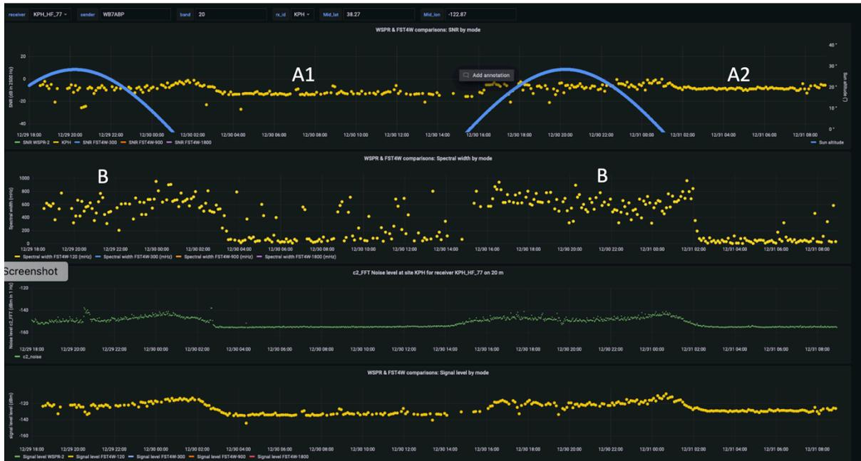
Figure 3.6. Time series of SNR with sun elevation, spectral spread, noise level and signal level for WB7ABP at KPH.
