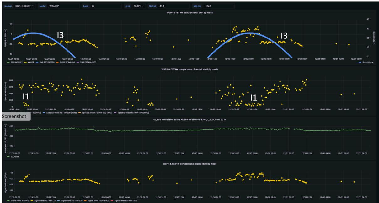
Figure 3.17. Time series of SNR with sun elevation, spectral spread, noise level and signal level for WB7ABP at KK6PR.
