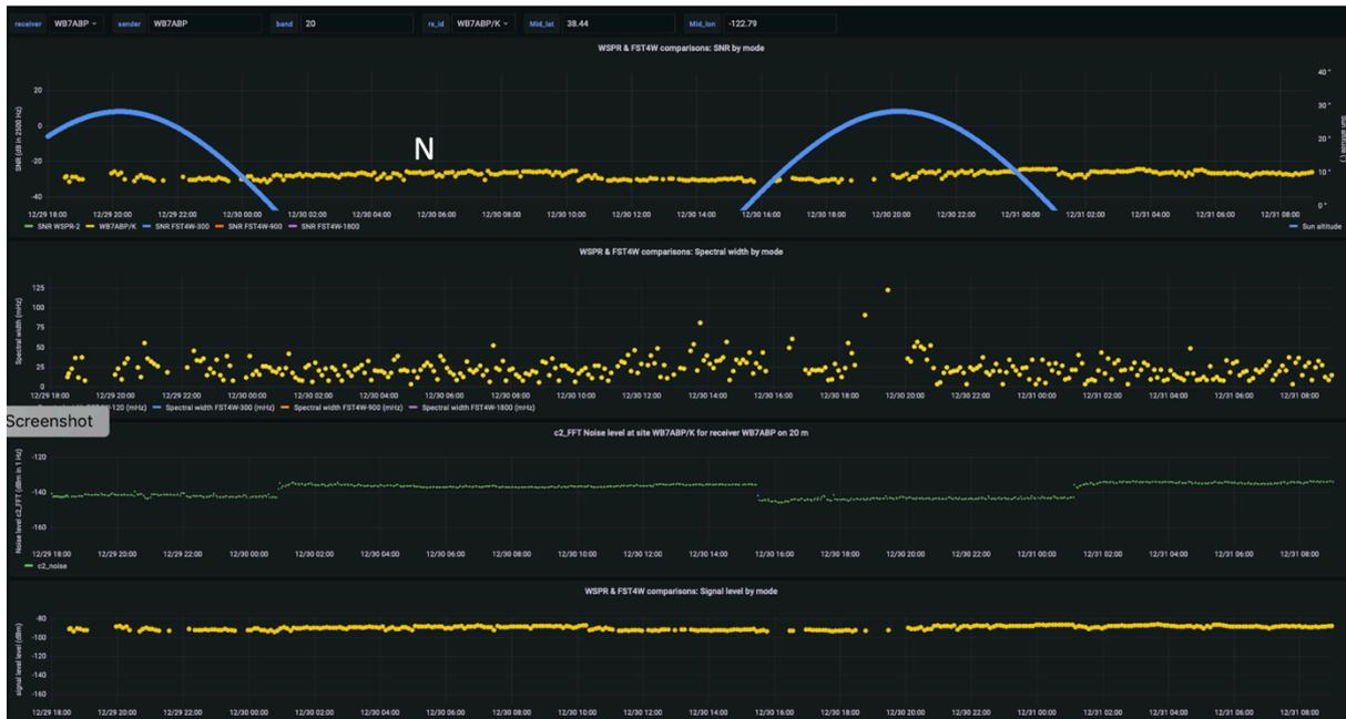
Figure 3.1. Time series of SNR with sun elevation, spectral spread, noise level and signal level for WB7ABP at same location reporting as WB7ABP/K.
