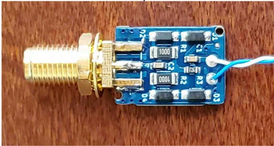
External 25MHz clock interface board. from WB6CXC
